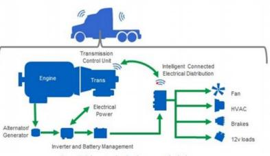
Figure 7. Schematic of a 48-volt commercial vehicle.
