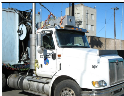
Figure 1: Truck with Portable Emission Measurement Equipment Installed
