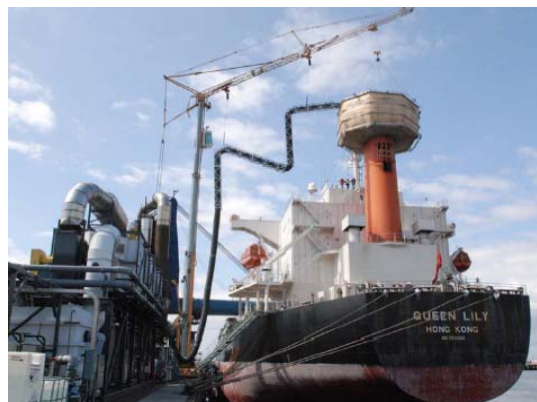
Figure 1: AMECS during Testing on the Queen Lily
