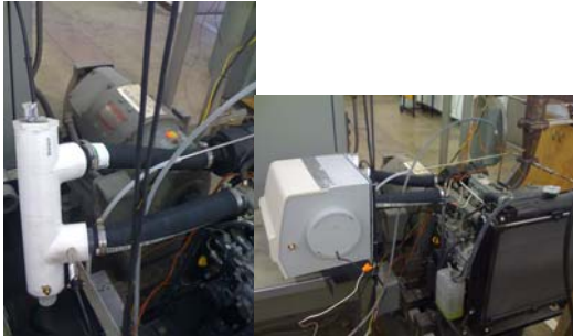
Figure 1: Diesel engine with the water atomizer unit (left) and humidifier (right)
