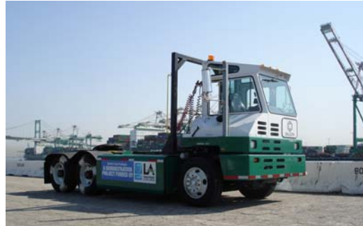
Figure 1: Heavy-Duty Class 8 Electric Truck in Demonstration
