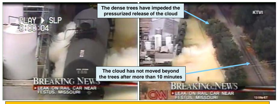
A Chlorine Leak from a Railcar Demonstrates the Effect Physical Structures Have on a Toxic Cloud's Speed of Travel
