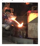
metal to cool and solidify, removing the mold or casting, degating, heat treating, surface cleaning, and finishing. Possible emission sources from such operations include, but are not limited to, fume, particulate, or dust from the melting, pouring, casting, degating, heat treating, coating, brazing, finishing, or surface cleaning
