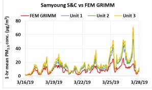
Coefficient of Determination (R<sup>2</sup>) quantifies how the three sensors followed the PM<sub>2.5</sub> concentration change by the reference instruments.
