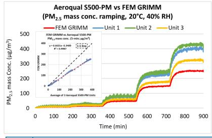
The Aeroqual S500-PM sensors showed very strong correlations with the corresponding FEM PM<sub>2.5</sub> data ( $R^2 > 0.99$ ) at 20 °C/40% RH.
