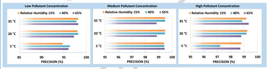
Overall, the Redspira sensors showed high precision for all the combinations of low, medium and high PM<sub>2.5</sub> conc., T, and RH.
