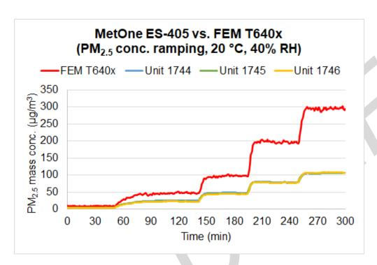
The MetOne ES-405 sensors tracked well with the concentration variation but underestimated PM<sub>2.5</sub> concentration values compared to the FEM T640x in the concentration range of 0 -300 μg/m<sup>3</sup>.
