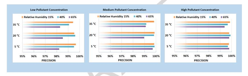
Overall, the three MetOne ES-405 sensors showed high precision for all combinations of PM<sub>2.5</sub> conc., T, and RH.
