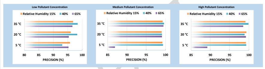
Overall, the Kunak sensors showed high precision for all of the combinations of low, medium and high PM<sub>1.0</sub> conc., T and RH except at medium and high PM<sub>1.0</sub> conc. under 5 °C/65% RH.
