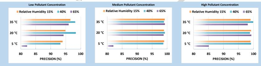
• Overall, the Kunak sensors showed high precision for all of the combinations of low, medium and high  $PM_{2.5}$  conc., T and RH except at 5 °C/65% RH for all  $PM_{2.5}$  levels
