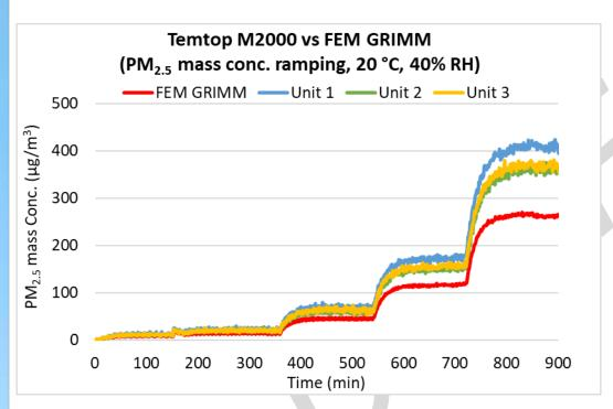
The Temtop M2000 sensors tracked well with the concentration variation as recorded by the FEM GRIMM in the concentration range of 0 - ~250 μg/m<sup>3</sup>.
