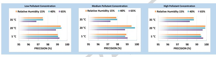
Overall, the Dylos DC1700-PM sensors showed high precision for all of the combinations of low, medium and high PM<sub>2.5</sub> conc., T, and RH.
