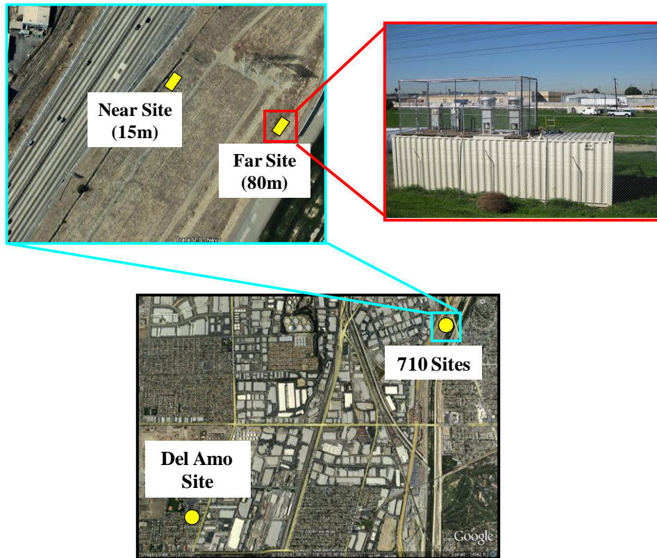
Figure 1 Aerial view of the sampling area showing the locations of the two monitoring stations near the I-710 freeway (“near” and “far” sites) with respect to the background site in Del Amo. An actual picture of the “far” site is also included
