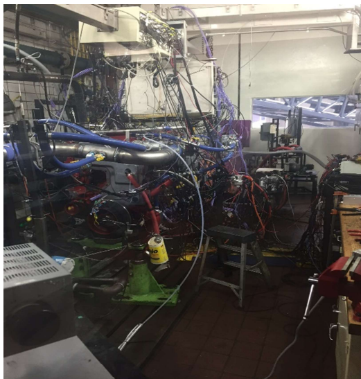
Figure 1: Test Engine on Dynamometer
