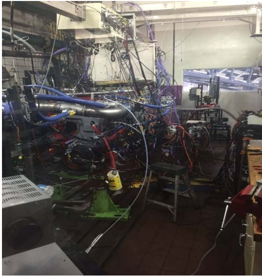
Figure 35: ISX15-G Ultra Low NOx Test Engine
