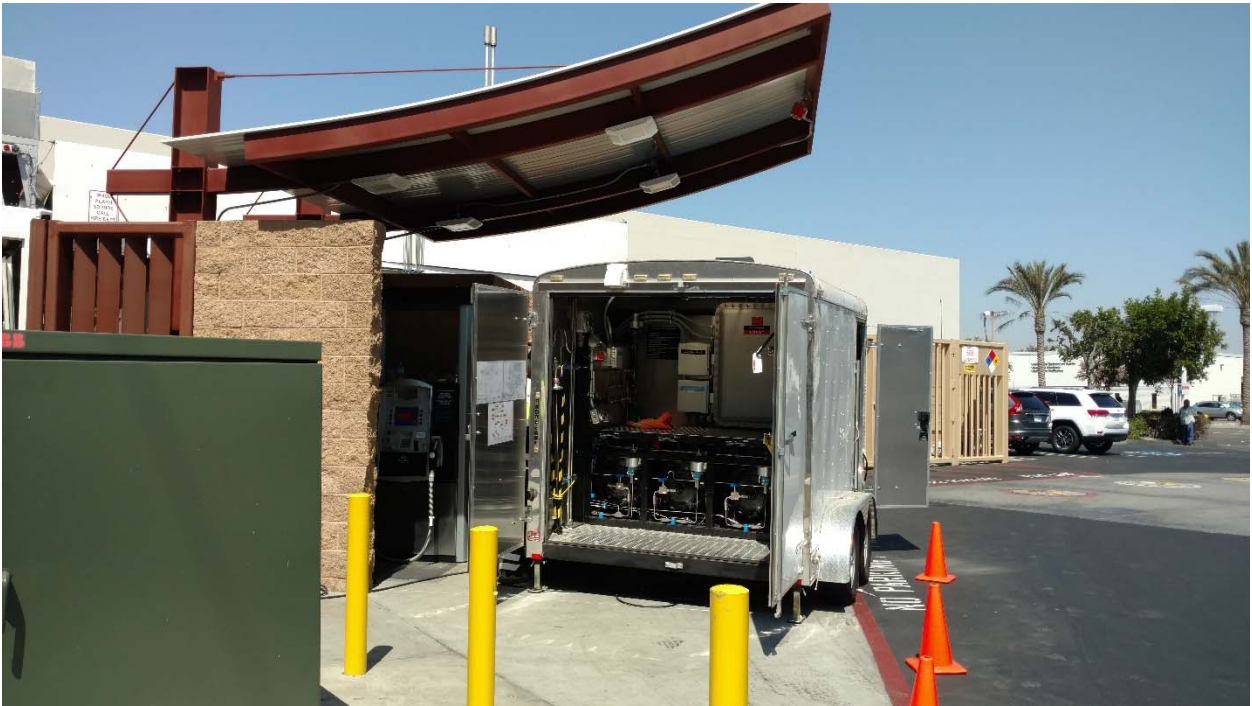
Figure 23: CDFA/DMS Testing Air Liquide System Co-located at Anaheim 76 station with NREL HyStEP Equipment
