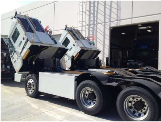
Figure 1: Upgraded Electric Yard Tractors
